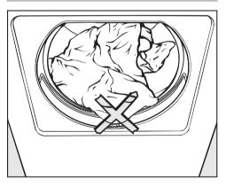
Before closing the door make sure the fluff filter is correctly positioned.
